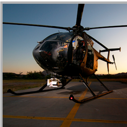
A Boeing Little Bird helicopter, equipped with sensor pods for autonomous flight.
