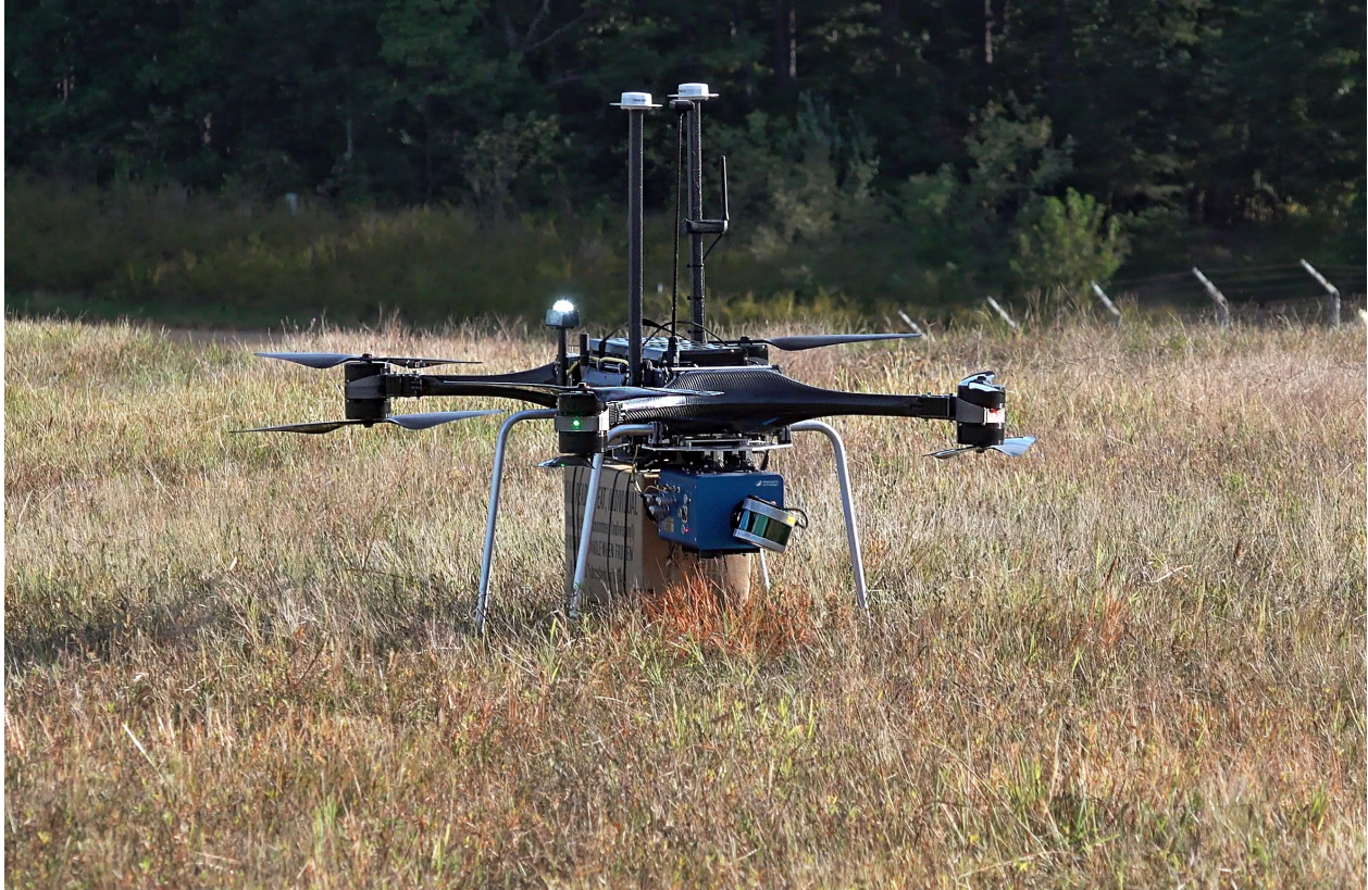
Near Earth Autonomy's system enables autonomous landing and cargo resupply
